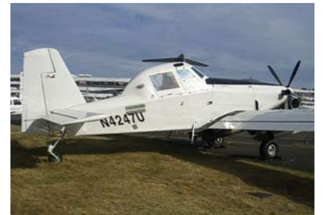
BELOW: The revival of the COIN attack aircraft? This Air Tractor AT-802U looks like something from a Mad Max movie but is a heavily armoured and armed modification of an agricultural crop duster. It has been evaluated by US Special Forces, and has at least one customer. It might offer an affordable alternative close air support asset in limited wars to today's high performance multi-role jets and armed UAVs. It can remain aloft for 10 hours and a second crew member can monitor a range of surveillance and targeting sensors from the roomy rear cockpit.
