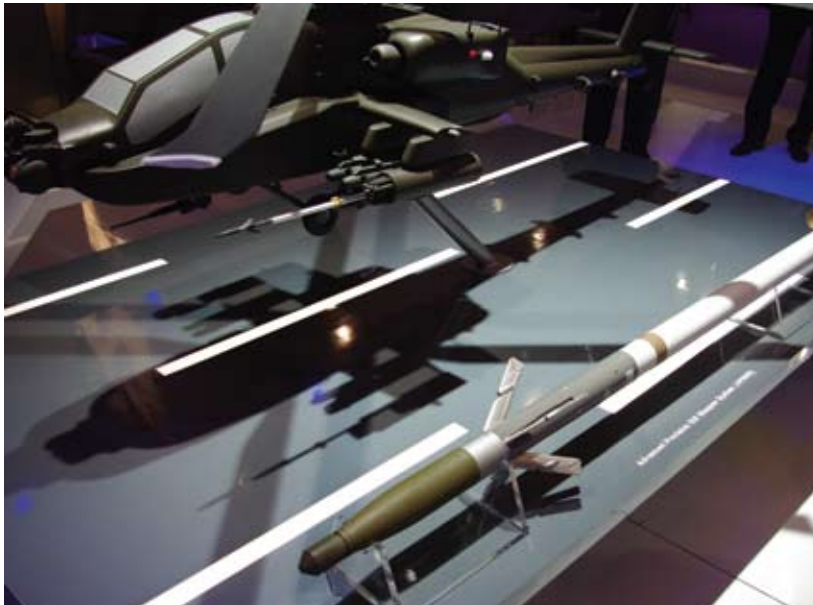
ABOVE - Unguided air-to-ground rockets, launched from helicopters or strike aircraft, are effective and powerful weapons, but cannot be used where there is the danger of causing collateral damage to innocent people. New developments include the fitting of lightweight laser-guided target seekers which transform each rocket in a pod into a precision guided weapon, at a cost that is a fraction of that for existing precision ground attack missiles.
