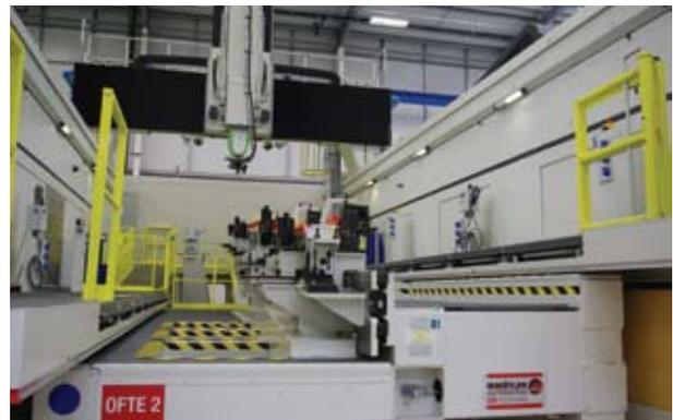
ABOVE - Automated assembly jig at GKN's new Bristol manufacturing facility for A350XWB composite inner wing spar production. (Editor's photo).
