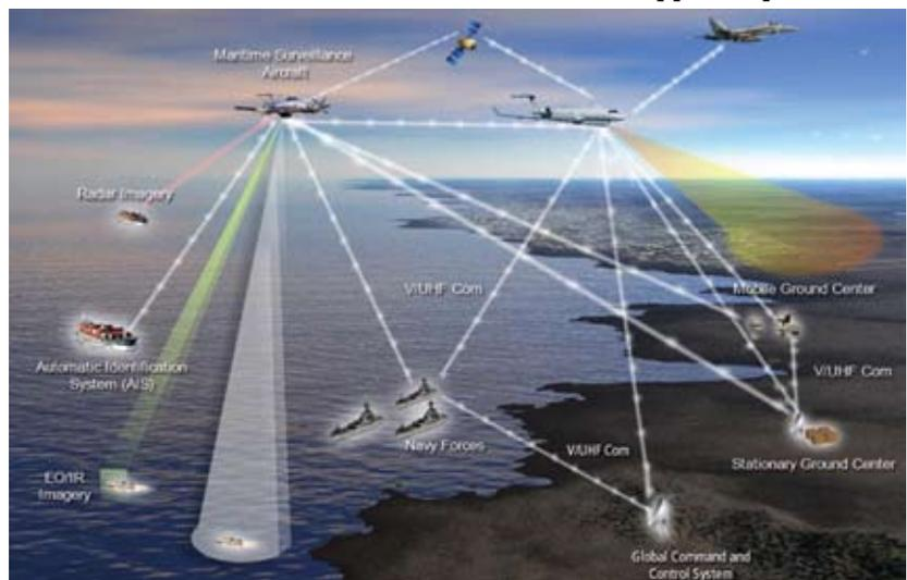
ABOVE - Schematic diagram showing how ISTAR air assets provide network connectivity. (Raytheon image)
