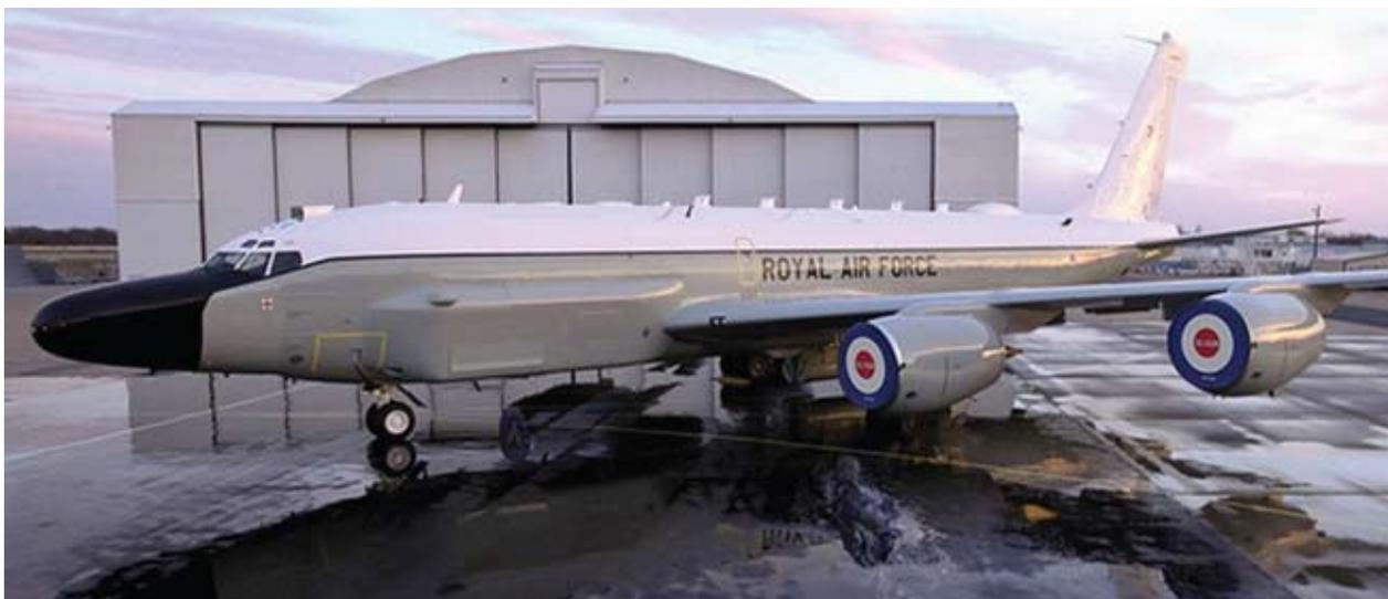
*ABOVE - The Boeing RC-135W Rivet Joint is a conversion from a KC-135 tanker and is the replacement for the Nimrod R1. (L3 image)*
