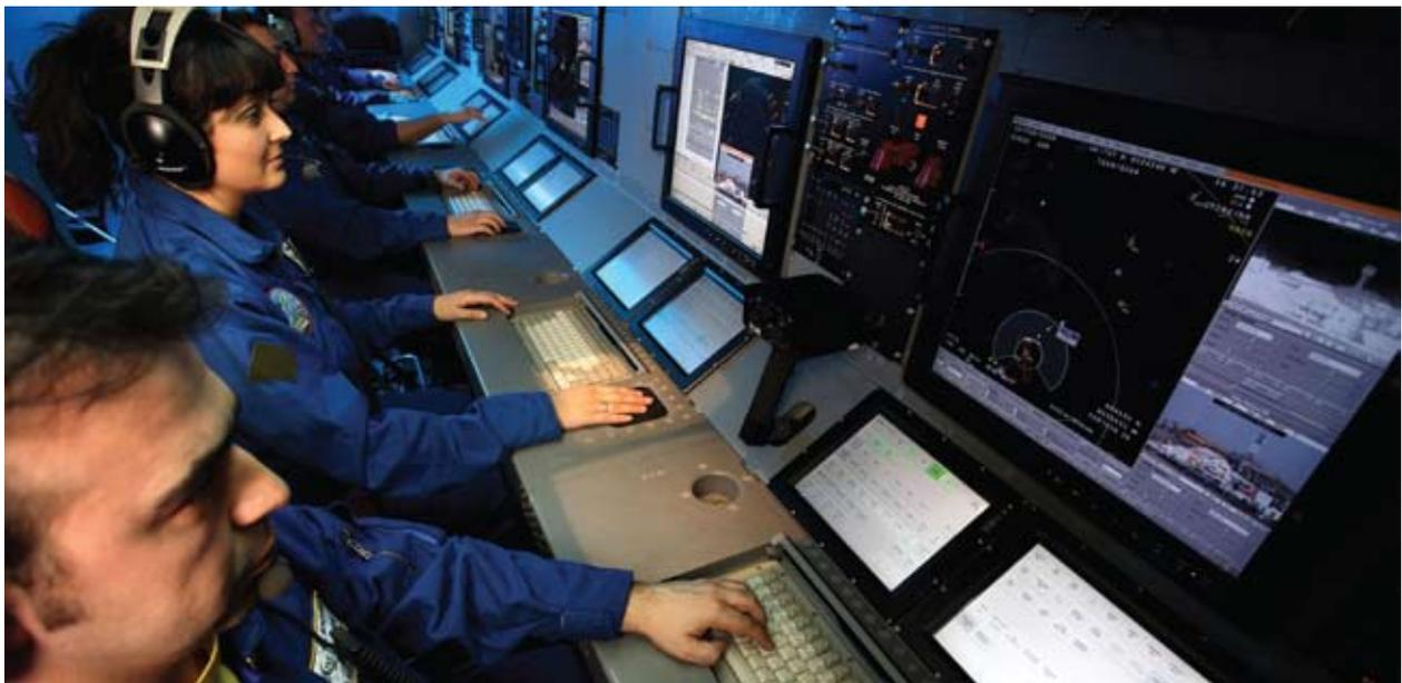
*ABOVE - Operators of maritime patrol aircraft, such as in this modernised P-3C Orion, can draw on a range of optimised sensors, from synthetic aperture radar, capable of detecting a periscope in high sea states, enhanced vision electro-optical turrets, sonar systems and exhaust and magnetic anomaly detection, in the search for surface targets or submerged submarines.*
