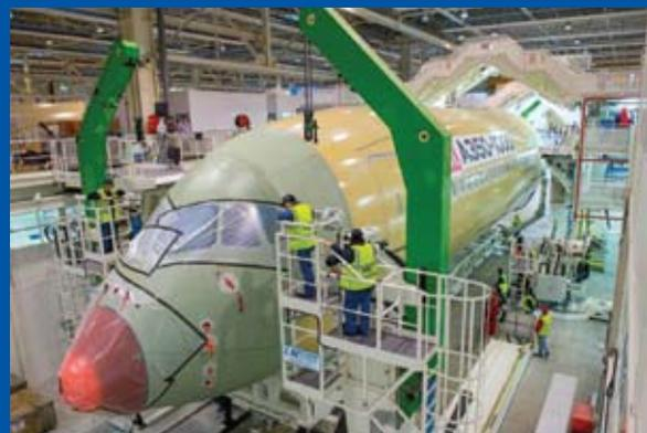
*ABOVE - Airbus has started the assembly of the first stretched A350-1000 which can carry up to 366 passengers in a typical three-class cabin layout, and can fly non-stop for almost 8,000 nautical miles. To date, 181 A350-1000s have been ordered by 10 customers. (Airbus photo)*
